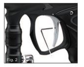
The Trigger's forward travel and over travel are fully adjustable so that the user can fine-tune the trigger to his/her exact preference.
