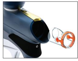
eyes are dirty. This is an extremely reliable system as long as the eyes are kept clean. The most common reason for dirty eyes is broken paint. If the eyes become dirty, the marker will default to a reduced rate of fire to prevent chopping. If this happens during game play, you can bypass this by turning the eyes off. Clean the eyes as soon as possible.
