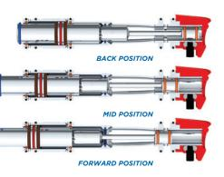
Air is supplied to the bolt at two points. A high-pressure supply of air is routed to the back of the bolt into the shot chamber. This air source is responsible for propelling the ball. Low-pressure air is supplied from the LPR to the solenoid. From the solenoid, the air is routed through two small holes to the section of the bolt referred to as the cylinder.
