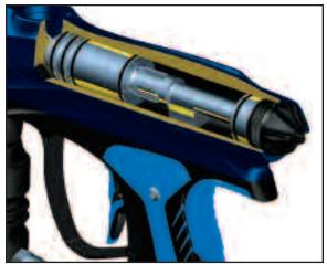
Back Cap out until it spins loosely. Now pull out the complete RAIL™ bolt kit from the PMR. To dis-assemble you unthread the front most part called the Can and the
